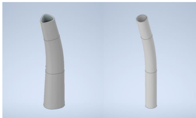
Figure 4. The initial part and the final part (used as mold) were created by Inventor
