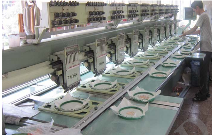
Fig 1. The studied computerized embroidery machine during operation in the industrial workroom
