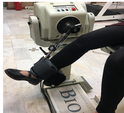
Figure 3. Stiffness measurement by biodex system 3
