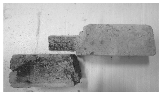
Figure 3. Failure surface of concrete beam strengthened with CFRP fabric in +20^{\circ}\text{C}
