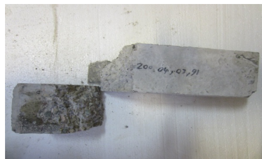
Figure 5. Failure surface of concrete beam strengthened with CFRP fabric in +80^{\circ}\text{C}
