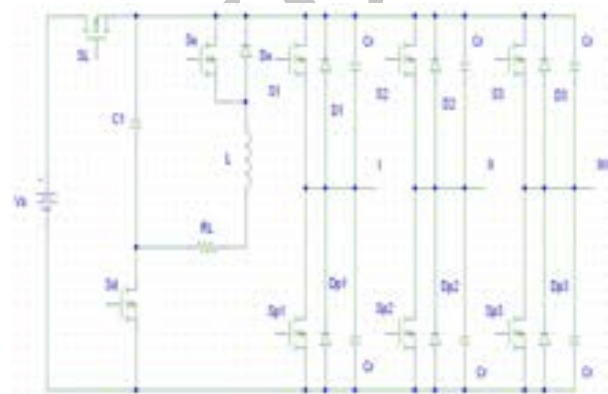
Fig. 3. New quasi DC Link inverter parallel with distributed link capacitor on the main switches
