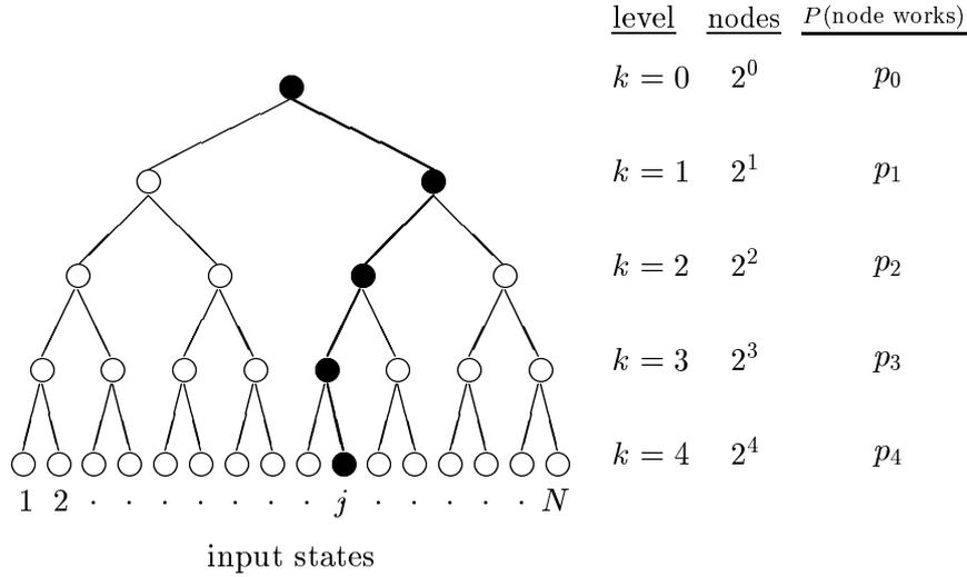
Figure 1: Binary tree-based model for a computer code.
