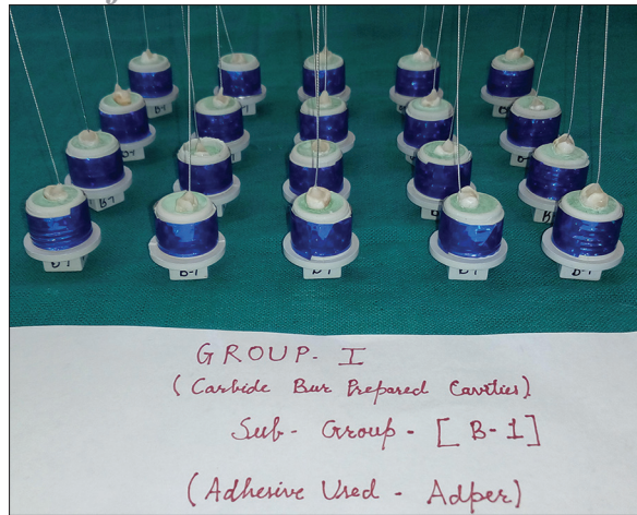
Figure 2: Photograph showing cavities prepared in Subgroup B1 – One-step self-etch (2-hydroxyethyl-methacrylate-free) adhesive system used on 20 teeth.
