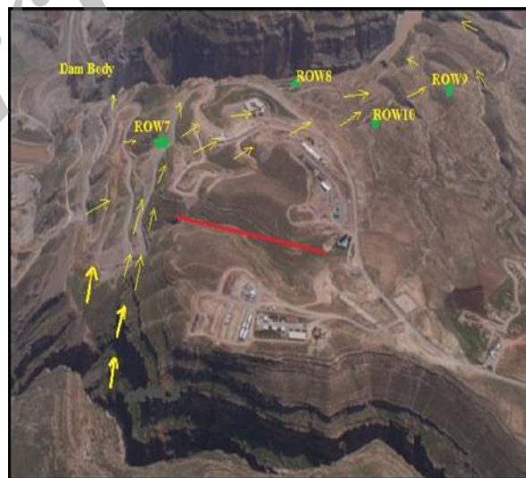
Figure 9. Seepage potential course (yellow arrows) and course without cross fractured to axis strike (red line)
