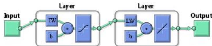
Figure 4. Neural network structure used with details
