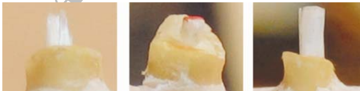
Fig. 2: Composite core fractured in group II and III in all specimens.
