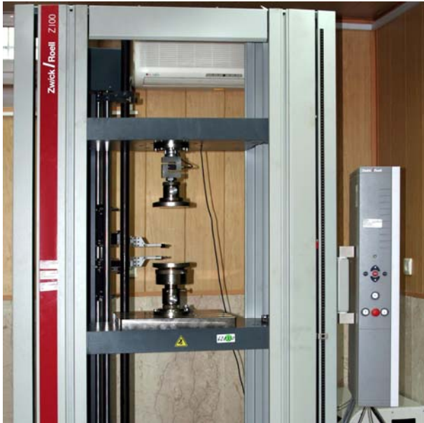
Fig 1. Zwick Universal Testing machine (Z/100, Germany) with a load cell of 50 KN and crosshead speed of 1 mm/min in mesiodistal direction.
