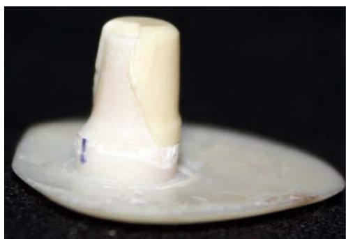
Fig (d1): Fracture area in chamfer
