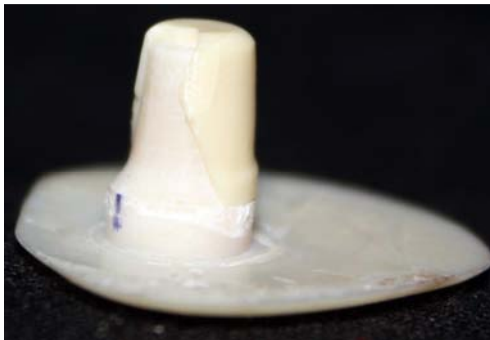
Fig (d1): Fracture area in chamfer
