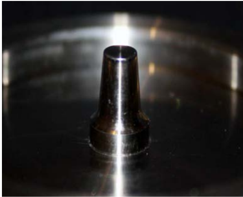
Fig (b1): Standard dies of Chamfer
