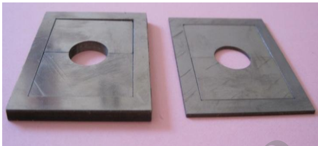
Fig 1. Two stainless steel molds, 13 mm in diameter and 1mm or 3mm height
