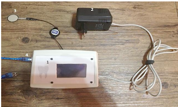
Fig. 1: Components of the bite force measuring device. (1) Body; (2) Power supply; (3) Sensor; (4) PC connector
