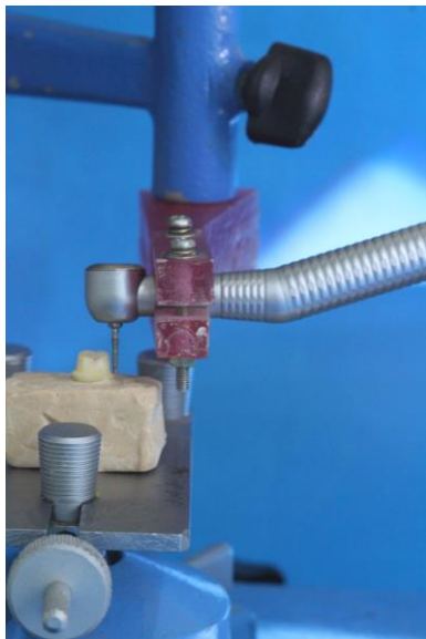
Fig. 1: The custom-made jig mounted on the surveyor
