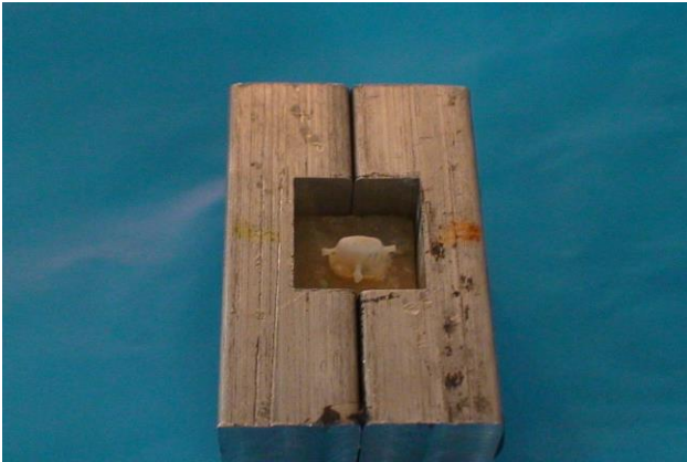
Fig. 3: Four wings were incorporated into the coping secured in a split mold
