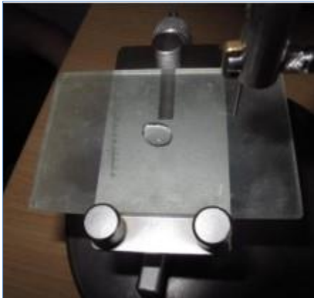
Fig. 1: The water-drop test
