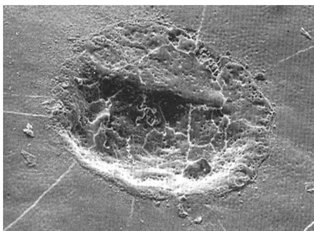
Figure 5. Human tooth melted with 100 pulses from a Ho: YAG laser (pulse duration: 3.8 microsecond, pulse energy: 18 mJ, 1 Hz) 2 .
