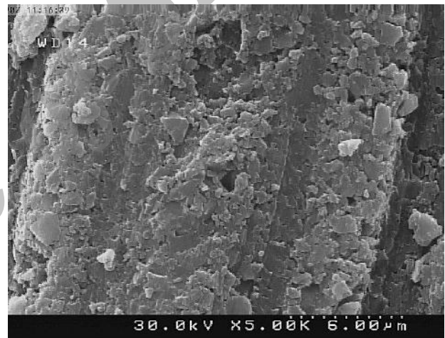
Figure 14. Surface treated by Bur (Original magnification \times 5000 , bar= 6\mu\text{m} )
