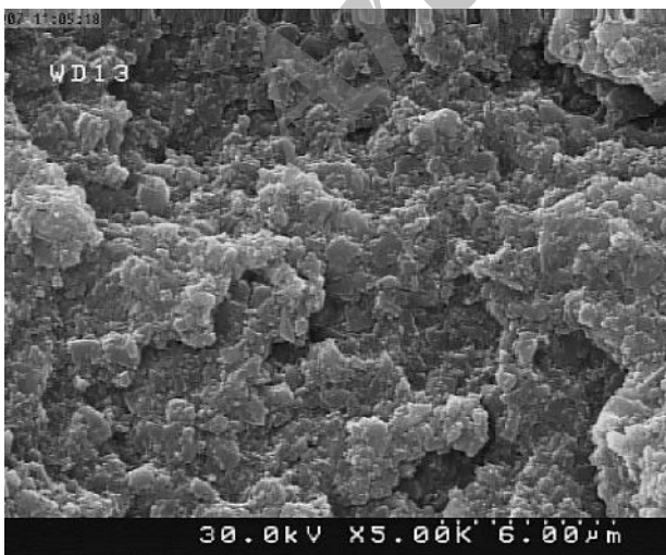
Figure 6. Surface treated by Er,Cr:YSGG laser with output power of 3 W (Original magnification \times 5000 , bar=6 \mu\text{m} )
