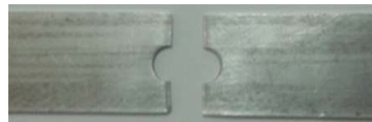
Fig.1 The fracture of the component with a hole in the tensile test
