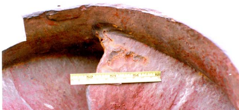
Figure 16. Cavitation erosion-corrosion of a centrifugal pump's impeller
