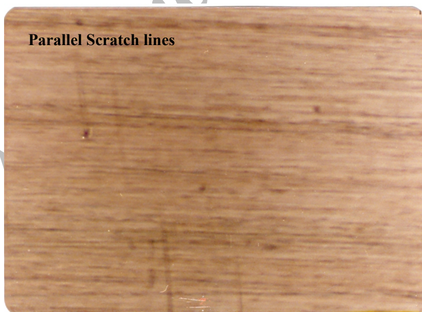
Figure 4. Original alloy surface finish before being cavitiated, alloy AISI 304 Mag. x 100
