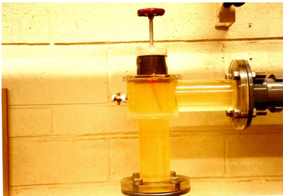
Figure 18. the constructed choke valve
