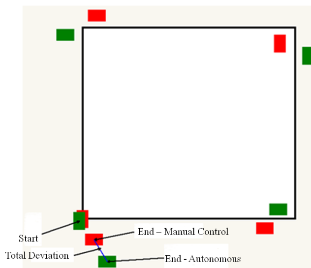
Fig.9. Robot testing in the 4x4 m square path
