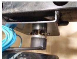
Fig.5. Rotary encoder mounted on rotating shaft
