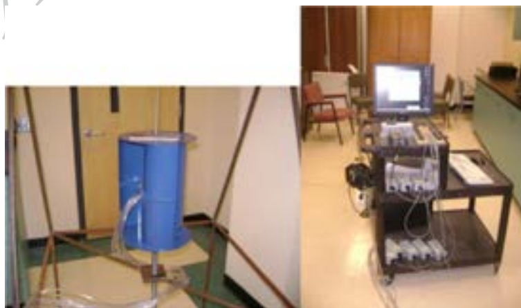
Figure 2 Setup of Savonius rotor model with pressure transducer data acquisition system for drag force measurement.
