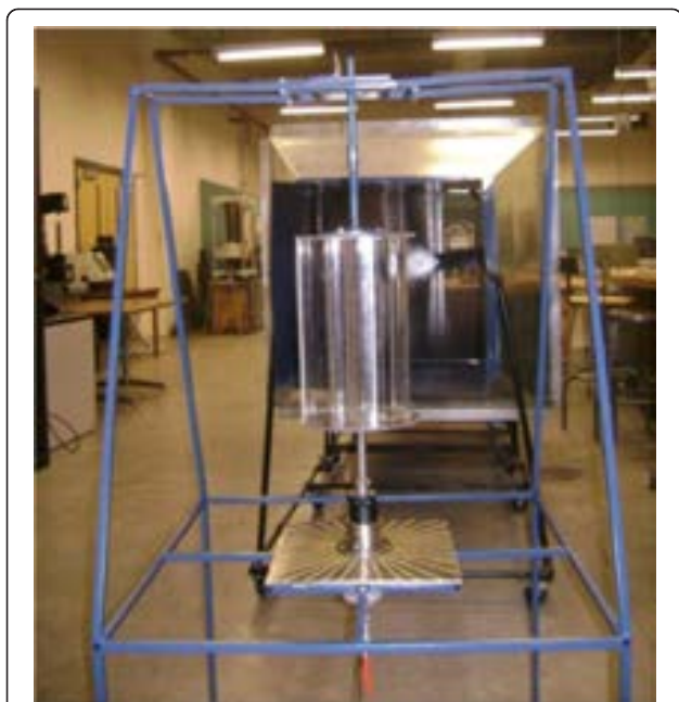
Figure 5 Setup of wind tunnel and Savonius rotor model for static torque measurement.
