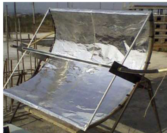
Figure 1 The fiberglass-reinforced plastic parabolic trough.
