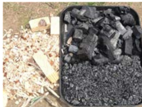
Figure 1 Representative raw yellow pine and resulting biochar from pyrolysis at 400°C.
