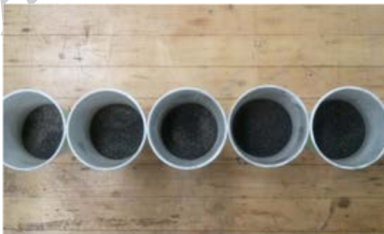
Figure 2 Representative prepared samples after sieving and mixing.
