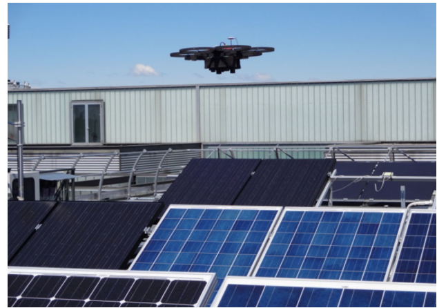
Fig. 5 PV modules inspection at Solar Tech Laboratory by Nimbus PPL-610 UAV platform
