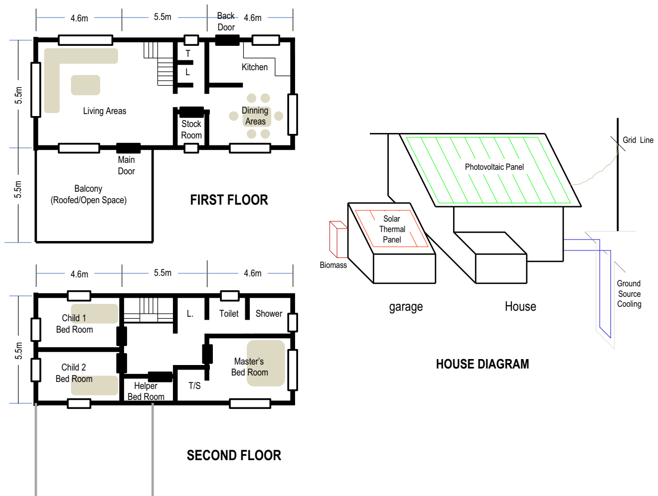
Fig. 8 House floor plan and schematic diagram for solar thermal, PV system, ground source cooling, biomass heater and grid-connected electricity
