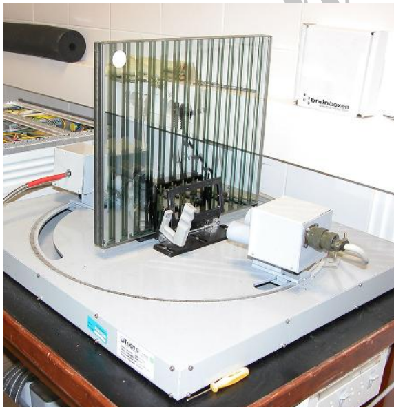
Fig. 8 UV-VIS-IR spectrometer to measure direct light reflection and transmission measured
