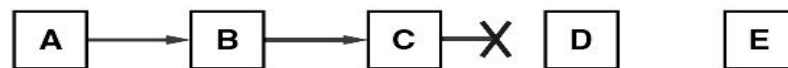
Fig. 4. Route maintenance example (Node C is unable to forward a packet from node A to node E over its link to next hop through D)
