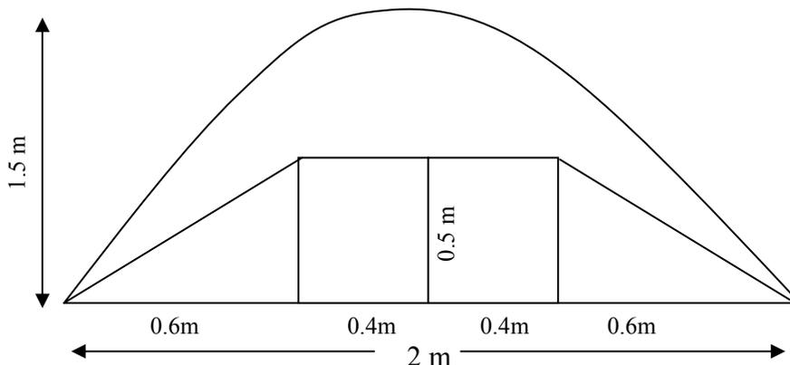
**Fig. 2:** Section of windrow system
