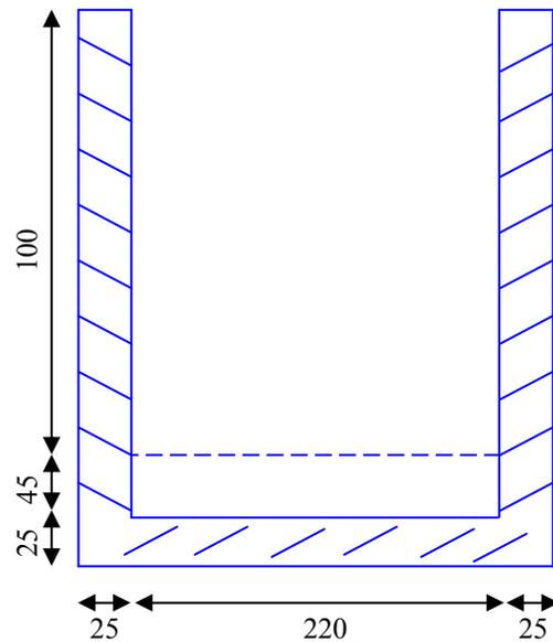
**Fig. 1:** Plan and cross section of pit system; dimensions are as mm
