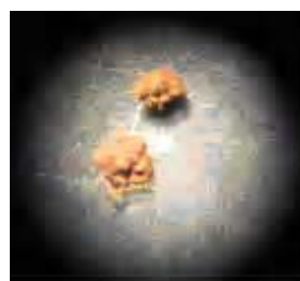
Fig. 2: Formed granules in UASB part of hybrid reactor
