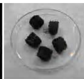
Fig. 3: Formed biofilm in UAFF part of hybrid reactor
