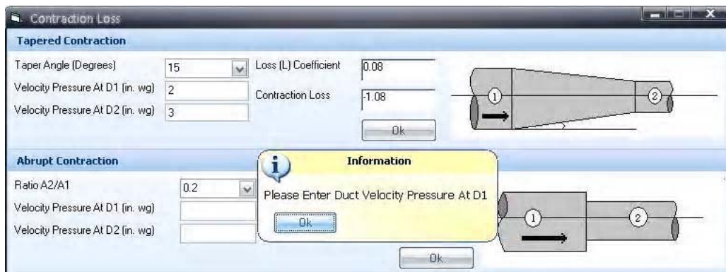
Fig. 8: Contraction and Expansion loss section
