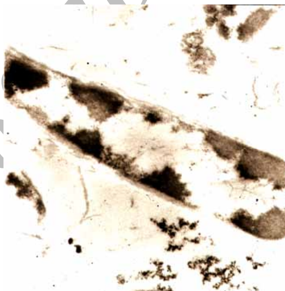
Fig.3D(x50000) It was striking to notice that the internal shards were composed of a linear arrangement of smaller nanocrystallites.
