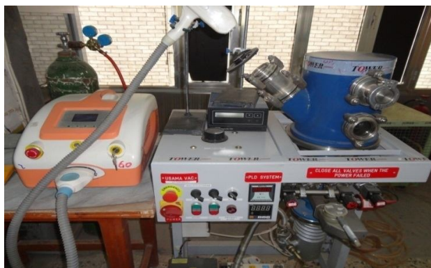
Fig. 1. PLD system Set-Up
