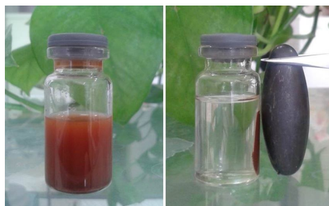
Fig. 5. Images of the ethanol solution (a) with dispersed magnetic \text{Fe}_3\text{O}_4@\text{SiO}_2 nanoparticles and (b) after applied magnetic field
