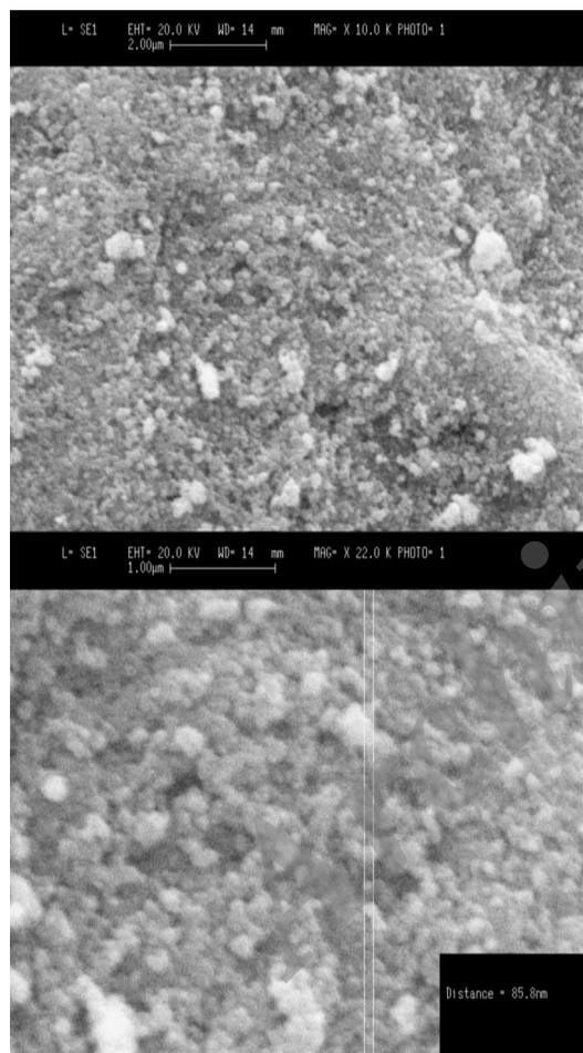
Fig. 4. SEM images of ZnO nanoparticles
