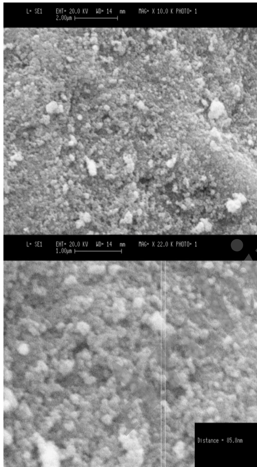
Fig. 4. SEM images of ZnO nanoparticles
