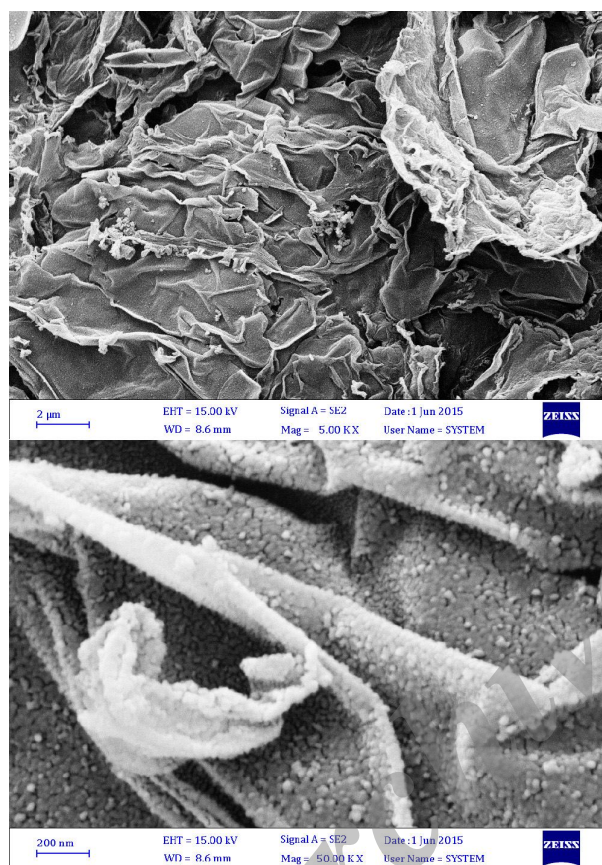
Fig. 7. SEM images of \text{SiO}_2 synthesized by oleic acid
