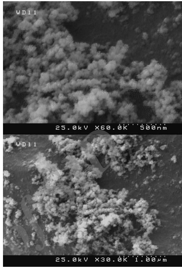
Fig. 6. SEM images of MgFe 2 O 4 -ZnO nanocomposite
