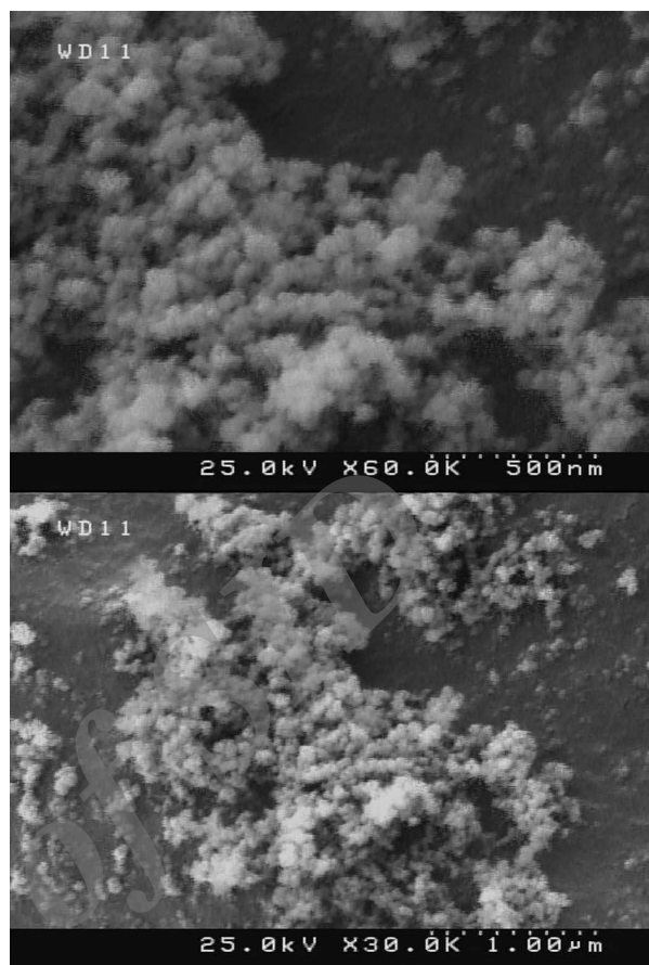
Fig. 6. SEM images of MgFe 2 O 4 -ZnO nanocomposite
