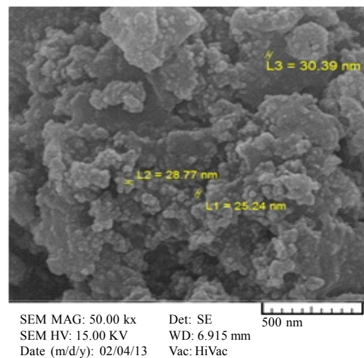
Fig. 4. SEM image of nanocomposite PVP: \text{SiO}_2 ; 2:3 in weight (sample 3)
