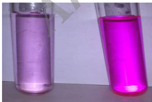
Fig 11. Rhodamine B after 100 minutes photodegradation in the presence of Fe 2 O 3 -TiO 2 nanoparticle
