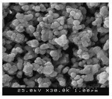
Fig. 4. SEM images of LCO NPs.
