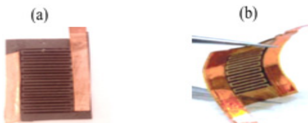
Fig. 9. (a) Optical image of MoS 2 /rGO micro-supercapacitor electrode, (b) an optical photograph showing the flexibility of the MSC electrode.
