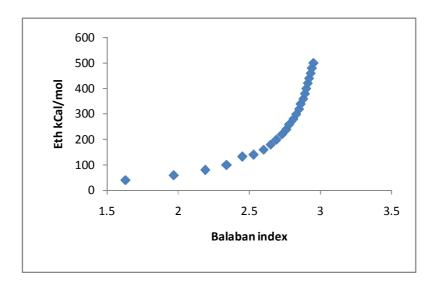
**Figure 3.** Plots of the Balaban index (J) versus thermal energy (E<sub>th</sub>) of 24 aldehydes.
