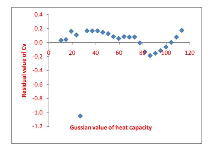
**Figure 9.** Plot of residuals against experimental value with Eq. (1) for the heat capacity of 24 aldehydes.
