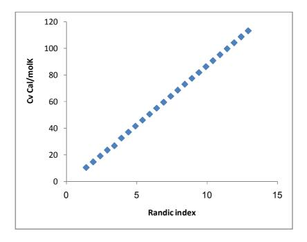
**Figure 1.** Plots of the Randić index  $(^1\chi)$  versusheat capacity  $(C_v)$  of 24 aldehydes.
