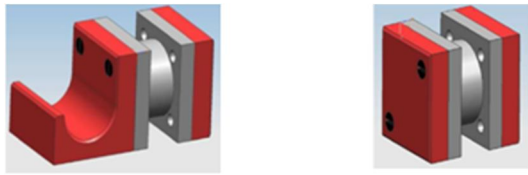
Fig. 8. Adapting of Coupling for friction fit and form fit
