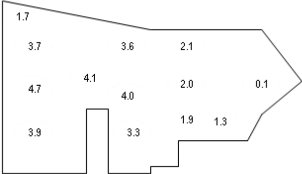
(a) Velocity field data at mid-face in m/s.
