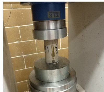
Figure 6. Uniaxial compressive test on a sandstone specimen with a strain gauge.
