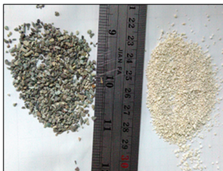
Figure 3. Sand and limestone particles from mesh 10 to mesh 30 and cutting size distribution.
