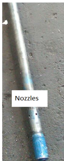
Figure 1. a) Drilling simulator with its diagram. Four nozzles b) and one cutting inlet are located on the right side and one outlet is located on the left side. c) The drilling fluid is pumped through the drill pipe and then comes into the annulus with the nozzles to remove the initial cuttings that are injected through the cutting inlet.
