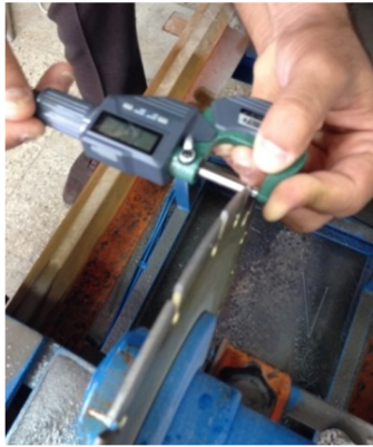
Figure 6. Digital micrometer for measuring saw wear.
