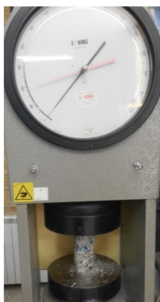
Figure 4. Uniaxial compressive strength test.
