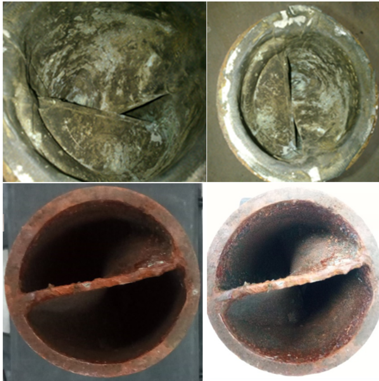
Figure 6. Static mixer of elliptical type (above) after 5 day with chocking and helical type (below) after 3 months without chocking.
