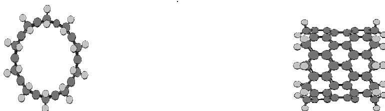
Fig. 1. Zigzag carbon nanotube (10-0).
