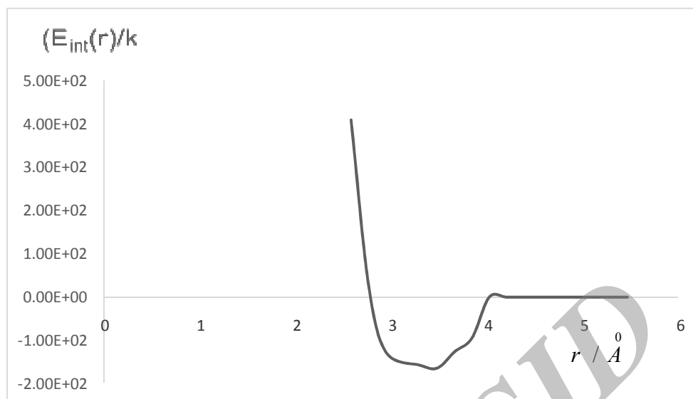
Fig.6. Plot of " E_{int}(r)/k " versus separation, r , for " CO_2 : C O_2 " system.
